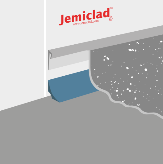
Self-coved with cove former & capping seal
